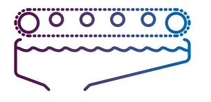
This prevents disruptive substances from concentrating and leading to subsequent problems such as breaks or deposits. Fines and fillers are coagulated in a way that retention on the wire is made possible.
